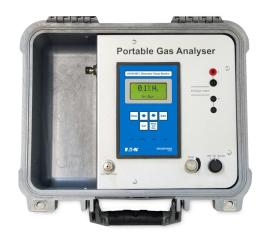
**Dual-gas measurement is provided by the KG6050.** It combines the measurement abilities of the K6050 with oxygen measurement by electrochemical cell. Concentration ranges from 100ppm to 100% of oxygen are available, depending on the application.
