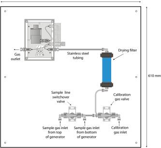
Electronics unit in optional EEx d enclosure with remote keypad
