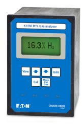
**The K1550 range of analysers** are ideal for measuring the % level of one gas in a binary or pseudo-binary mixture. For example, air is composed of many gases but in known, fixed ratios, therefore hydrogen in air is a pseudo-binary mixture and can be measured with the K1550.
