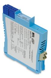
**The 9491-PS Power Supply** is the preferred method for supplying the 9460-ET range of intrinsically safe Ethernet modules and is based on an isolating power supply. It takes a 24V DC safe area / Zone 2 / Division 2 supply and produces an intrinsically safe, 12V DC nominal output capable of powering the Ethernet modules mounted in a Zone 1/ Division 1 hazardous area. The 9491-PS may be mounted in a safe area, Zone 2 or Division 2 hazardous area.
