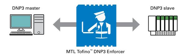
The MTL Tofino™ DNP3 Enforcer Loadable Security Module (LSM) is a plug-in Deep Packet Inspection (DPI) module providing Advanced Cyber Threat and Vulnerability Protection for DNP3 Protocol Communications making sure that the only DNP3 commands your control devices receive are approved commands from authorized computers.
